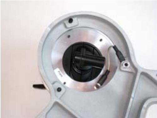
9. While holding the main bearing assembly upside down, carefully withdraw the slotted aluminum base/shaft from the bronze housing taking great care not to lose the thrust ball that resides inside. Put the bronze housing aside, again being careful not to let the thrust ball roll out.
