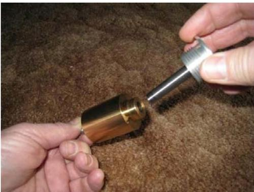
10. From underneath the metal chassis, insert the spindle into the threaded center hole of the metal chassis and screw the slotted base fully home. Using a large coin inserted into the slot underneath, tighten the bearing base as tight as you can to insure that it does not loosen over time as the platter rotates against it.
