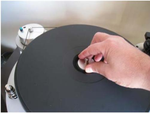
15. Fit the drive belt around the smaller 33 RPM groove in the motor pulley and in the lowest groove in the platter. (The lower pulley groove is for 45 RPM). Note: A 78 RPM-only pulley is available for listening to 78 RPM LP's.
