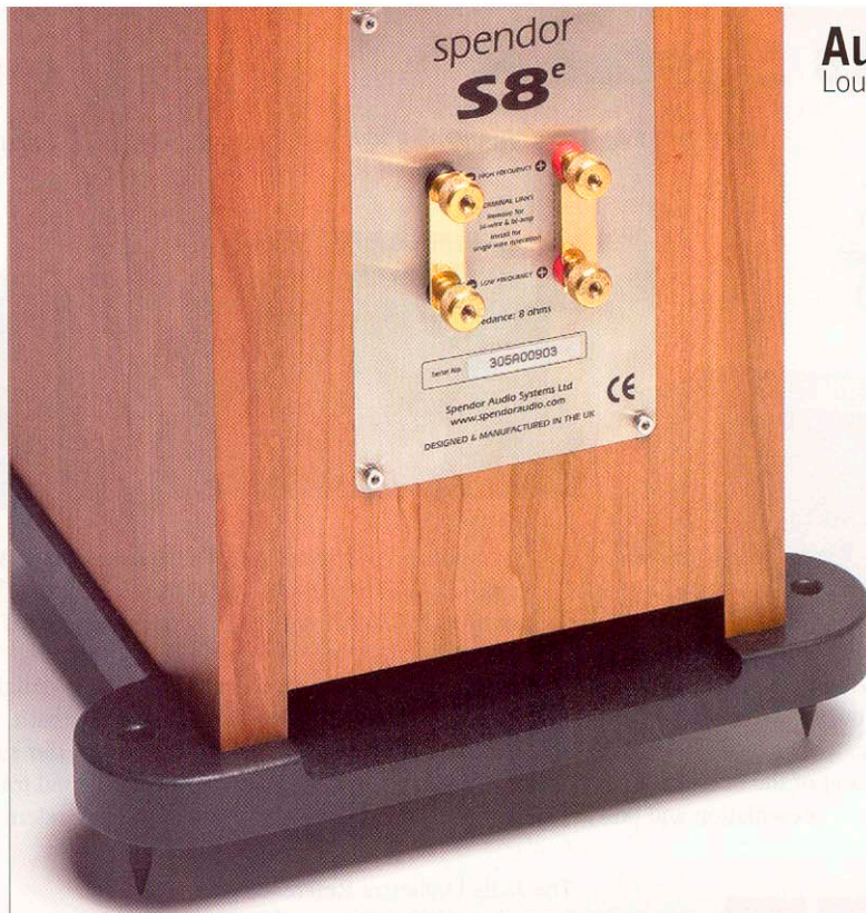
The substantial stainless steel terminal plate is secured to the cabinet via a damping membrane while the supplied heavy spiked plinth isolates the speaker's drivers from unwanted vibrations
